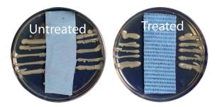
The Image above shows the results of an AATCC TM147 test (the light colored streaks are the bacterial organism). For the treated sample, the area of no growth at the sample edge is called the zone of inhibition and reported in millimeters. Some samples will not show a zone of inhibition, but the streaks will stop at the edge of the sample; as long as there is no growth under the sample, the result will be reported as a pass and is commonly referred to as contact inhibition.
